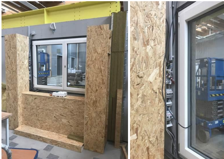
Figure 2.9 A “wall-simulator” attached to the sample of wall module that was used to simulate the critical details of connections between the module and existing building with integration of building services elements (left). The third version of switchbox designed to fit the gap between the hard part of the module and the existing building (right).
