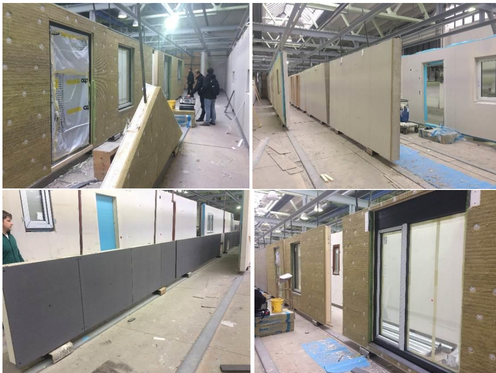
Figure 2.14 Prepared modules (standard wall, gable and base modules) for the Czech RLL in RDR factory before final production stage of integrated devices installation.
