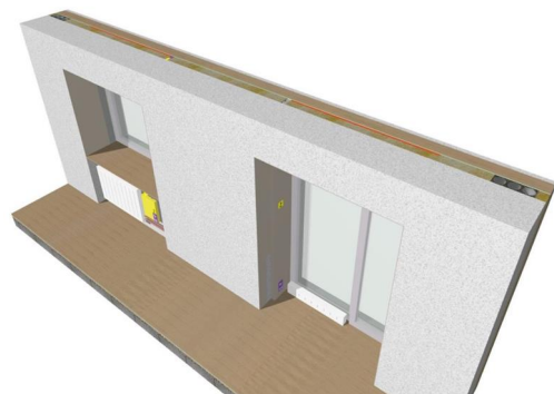
Figure 2.4 Final setting of the external wall module on the existing wall structure.
