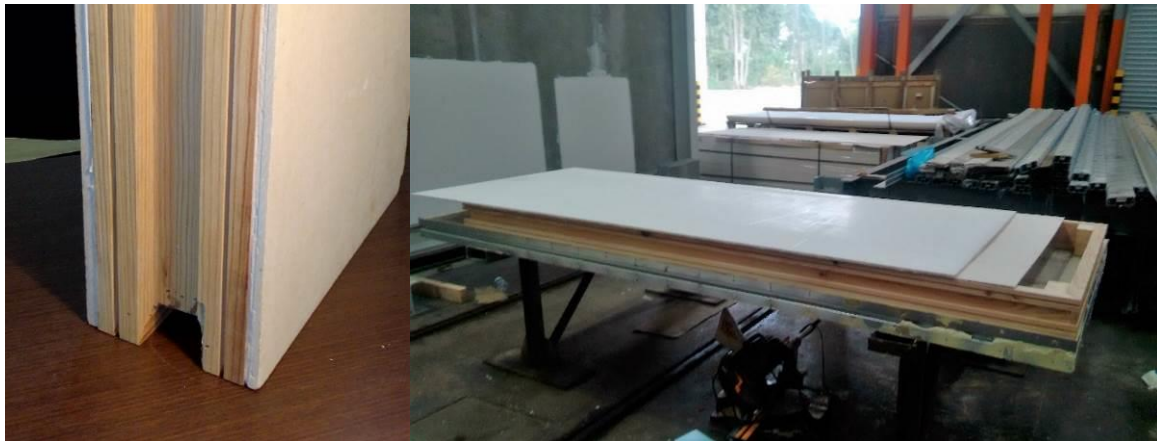
Figure 7.5 Prototype production (Frame detail and assembly process)
